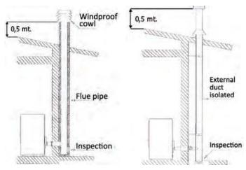
Fig. 2: connection to the flue pipe.
