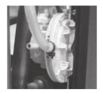
Pressure switch: monitors depression in the smoke duct. It is designed to shut down the pellet feed screw in the event of an obstructed flue or significant back-pressure in the presence of wind. At the time of the pressure switch will show "FLAR-DEP-FAIL".
