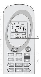
Keep the key TURBO (1) pressed for at least two seconds to activate this function. You will read the word "TURBO" (2) on the display of the remote control. Set temperature and working power will disappear. Press SEND (3) to transmit the selection to the pcb.
